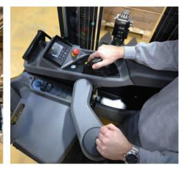
Ergonomic controls help to provide comfort, job satisfaction and productivity – while helping to minimize stress, strain and fatigue. They also include a fully adjustable (up/down, forward/back) steering console, for an optimized driving position and armrestmounted features for simultaneous control of drive and hydraulic functions.
